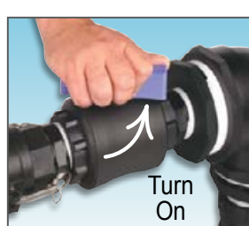
Step 8. Re-connect the Drag Hose to the Adaptor Set and turn on the Isolating Valve to begin irrigating at the new location.
