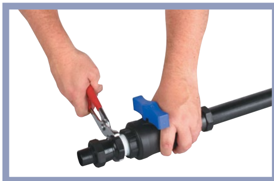
3. Do not over tighten. The recommended way to assemble a Ball Valve is finger tight. Tighten until firm with spanner or pipe grip. One to two turns should be all that is required.
