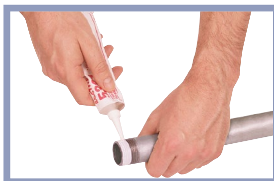
1 (b) thread paste sealant. The right sealant for threaded joints is non-hardening, compatible with plastic and doesn't add slipperiness to encourage over-torquing.
