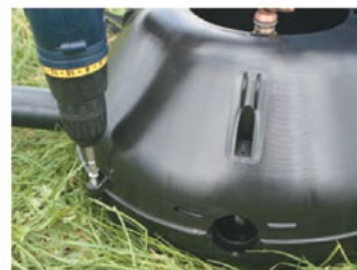
Secure top body by screws around the base.
