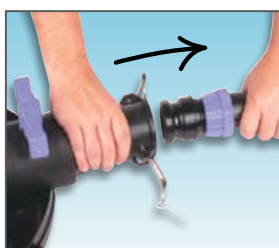
Step 3a Disconnect the Sub Main from the Drag Hose.
